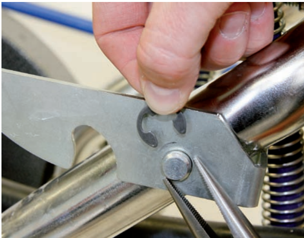
Removing the snap ring using snap ring pliers
