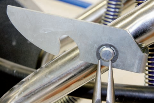
Insert the pin through the frame and adapter and fit the snap ring
